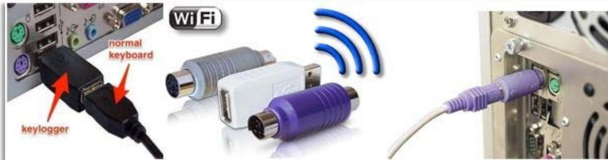
*Figure 1: USB, PS2 Hardware Keyloggers*
