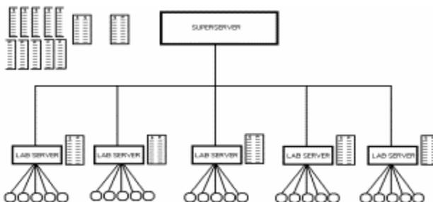
At the top level is the Superserver. Below this, at the intermediate level are the Intermediate Servers, and finally at the lowest level are the Client Nodes. Each of these is described below.
